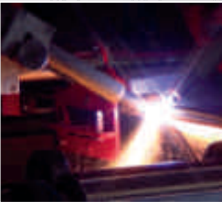
Combined Beveling unit: milling & Plasma process Cianfrinatrice simultanea anime
