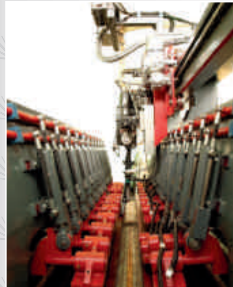
Water cooled copper backing bar Backing con barra in rame raffreddata ad acqua
