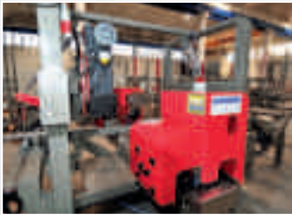
Combined Beveling unit: milling & Plasma process Cianfrinatrice simultanea anime
